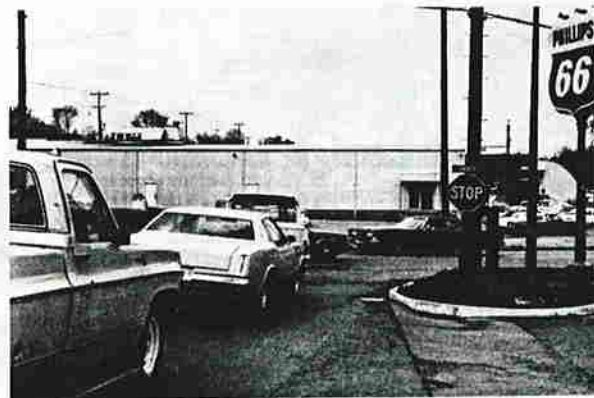
Delay to stopped approaches is the basis for level of service definitions.
