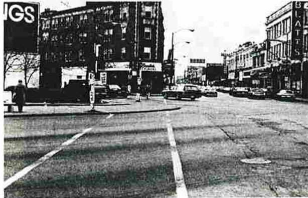
Elimination of multi-leg intersections through street closures greatly simplifies the operation of the intersection.
