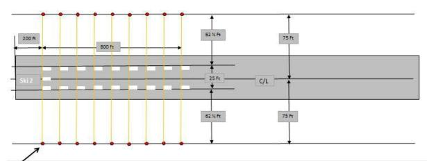
The red dots indicate the location of a pipe 75 feet off centerline adjacent to the start of each painted block. A one foot long piece of ½ inch pipe is installed in the ground at each location. With these pipes in place just run a long tape measure (yellow line) across the runway from pipe to pipe to find the end of your painted block. Measure in 62 ½ feet from each pipe to find the out side edge of the painted block, an additional 2 feet will mark the other side of the block.
