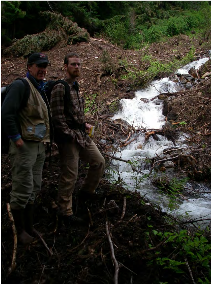
DF20. View east/upslope at debris channel. Stream is poorly channelized as a result of a high sediment/debris supply.
