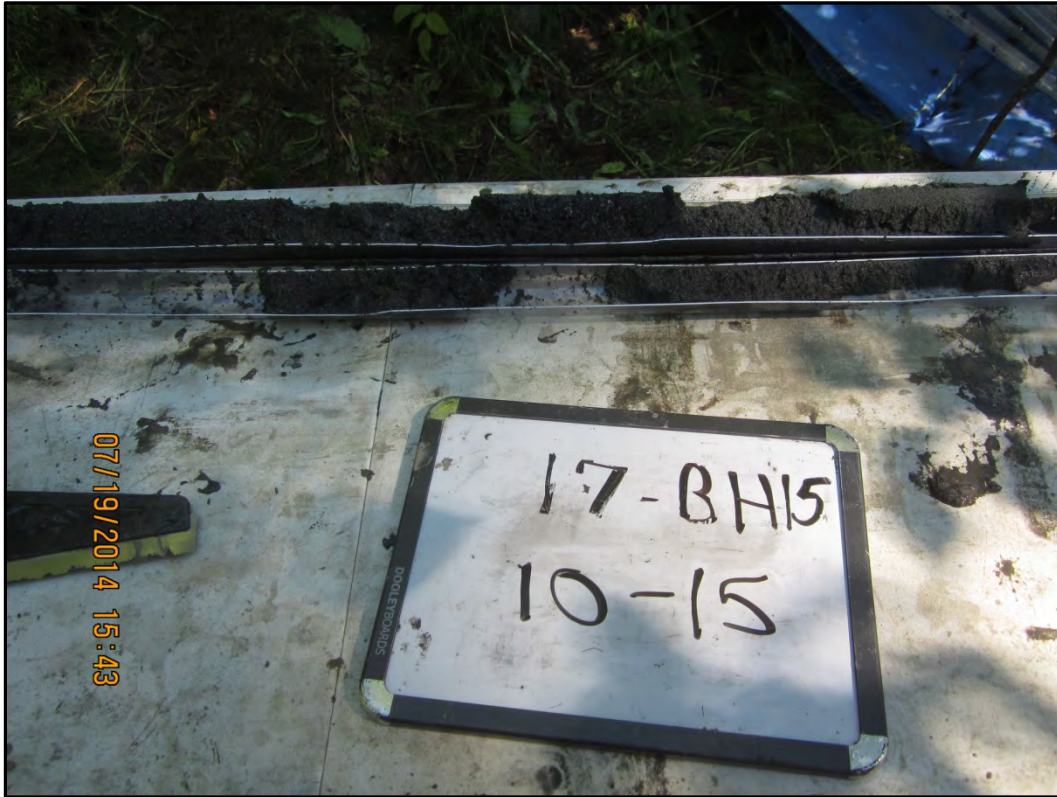
Photograph 7 – Soil lithology from boring 17-BH15 between 10-15 feet bgs. Sand with trace amount of silt, saturated. PID readings up to 140 ppm; sample collected from 14-15 feet bgs.
