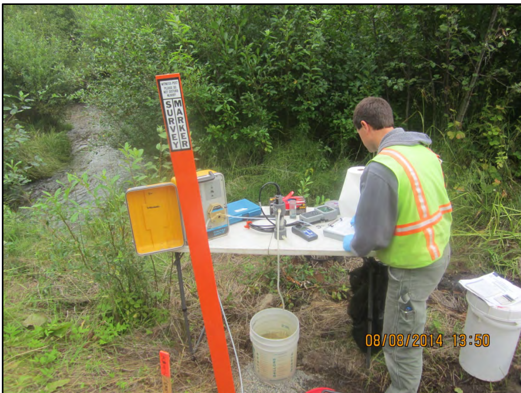
Photograph 30 – Groundwater sampling at 19-MW3 during the August re-sampling event, Horse Farm Creek in the background/left. View to the south-southeast.
