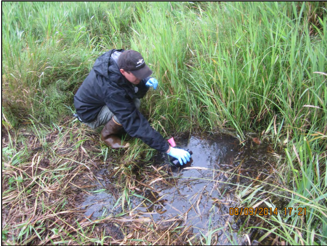
Photograph 13 – Collecting surface water sample 17-WS3 (co-located with sediment sample 17-SE6) sample using a new unpreserved sample jar. View to the west.
