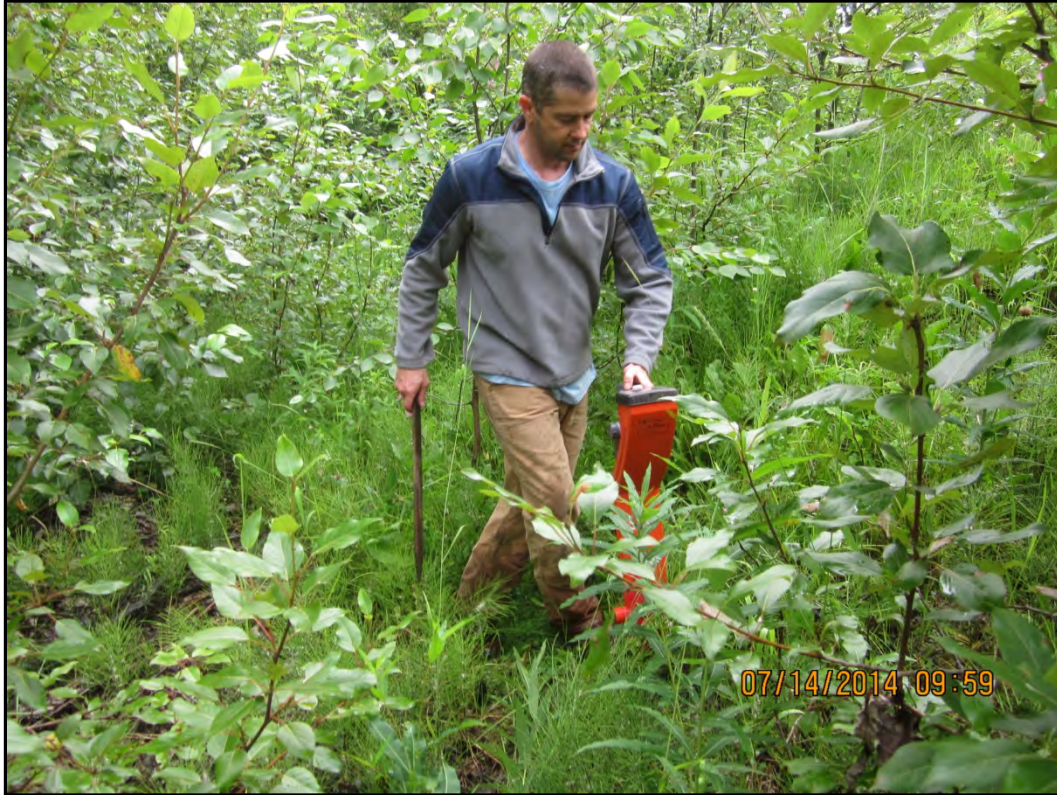
Photograph 39 – IPEC Utility locates conducted at PMP 25.5. IPEC and AP&T located utilities at all sites where work was performed in 2014.
