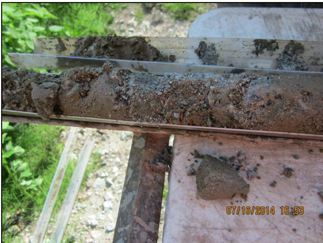
Photograph 26 – Close-up soil lithology from boring 19-BH12 between 5-10 feet bgs.
