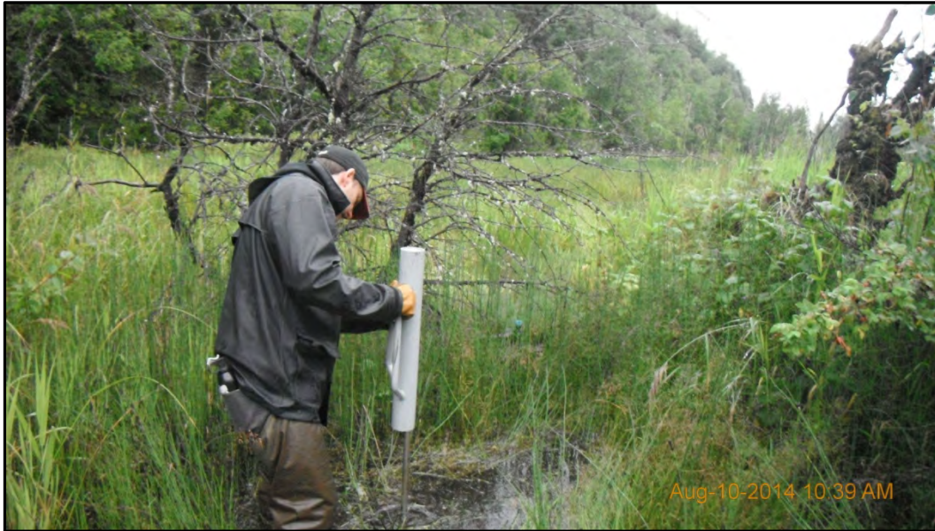
Photograph 15 – Hammering down sediment sampling equipment at 17-SE17. Some locations were picked if they had dead trees nearby. View to the southeast.
