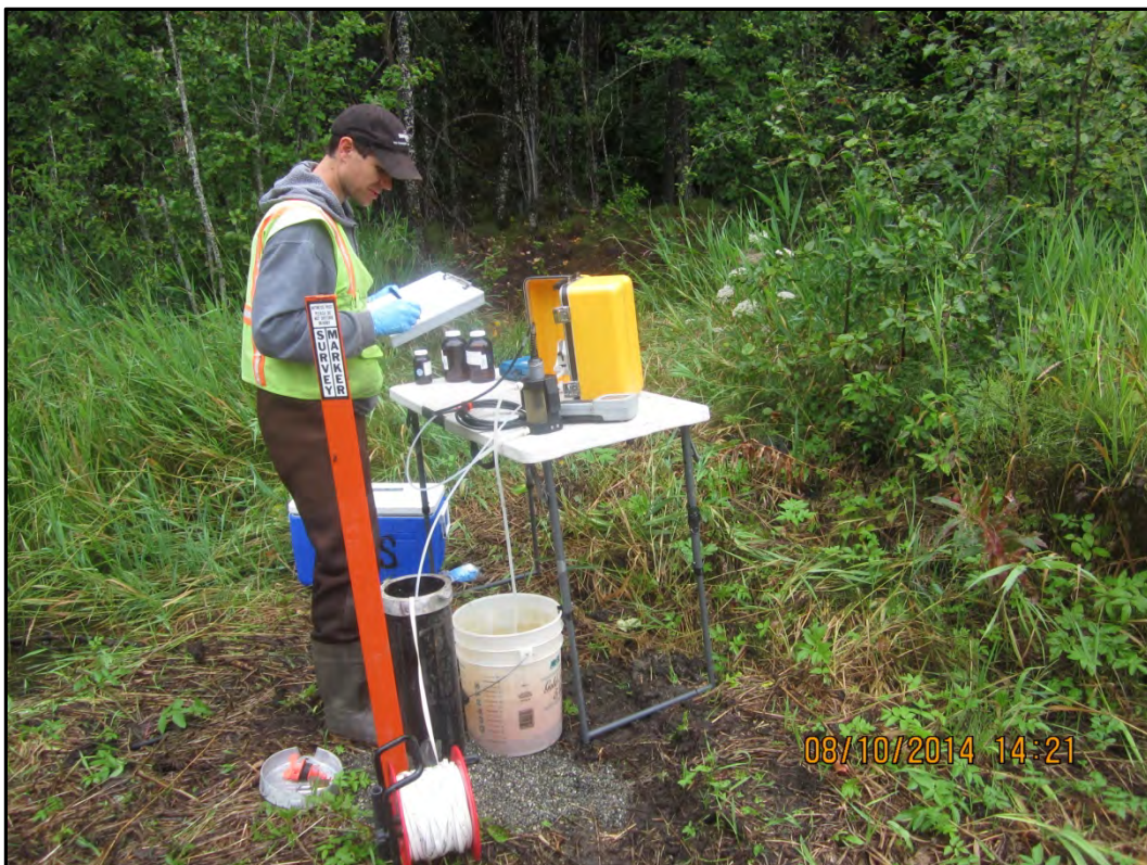
Photograph 10 – Collecting parameters prior to groundwater sampling at well 17-MW2 during the sample re-collection on August 10, 2014. View to the northeast.
