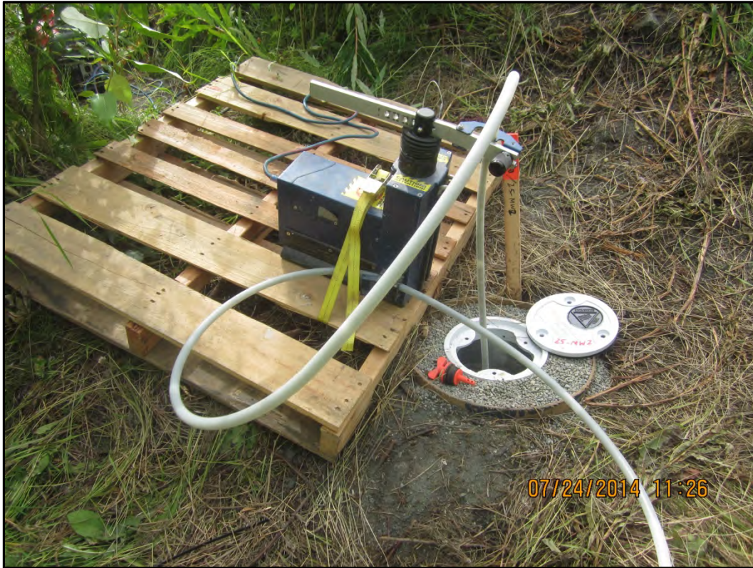
Photograph 51 – Developing well 25-MW2 with a Waterra inertia pump. Wells were also surged with a steel surge block prior Waterra development.
