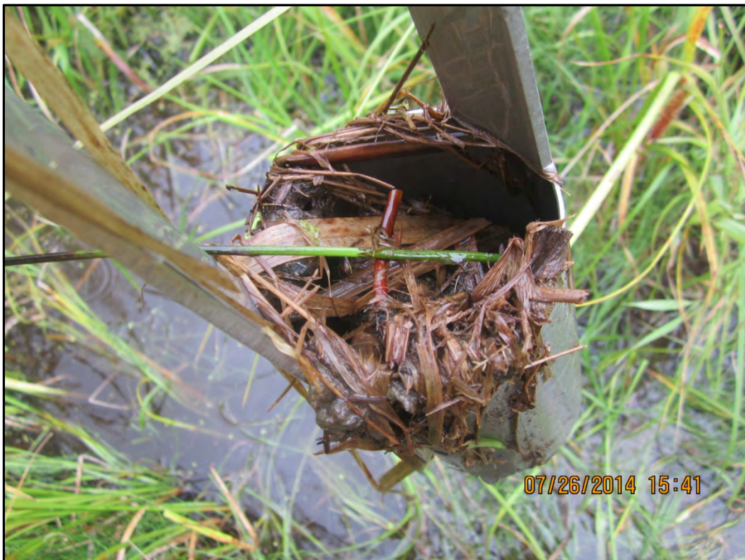
Photograph 16 – All wetland sediment samples contained swamp grass organics on top of the sediment.
