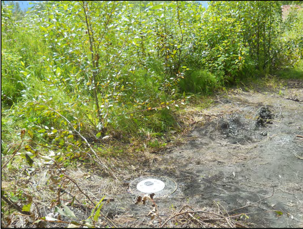
Photograph 49 – Upgradient well 25-MW6 completed along access road. View to the west.
