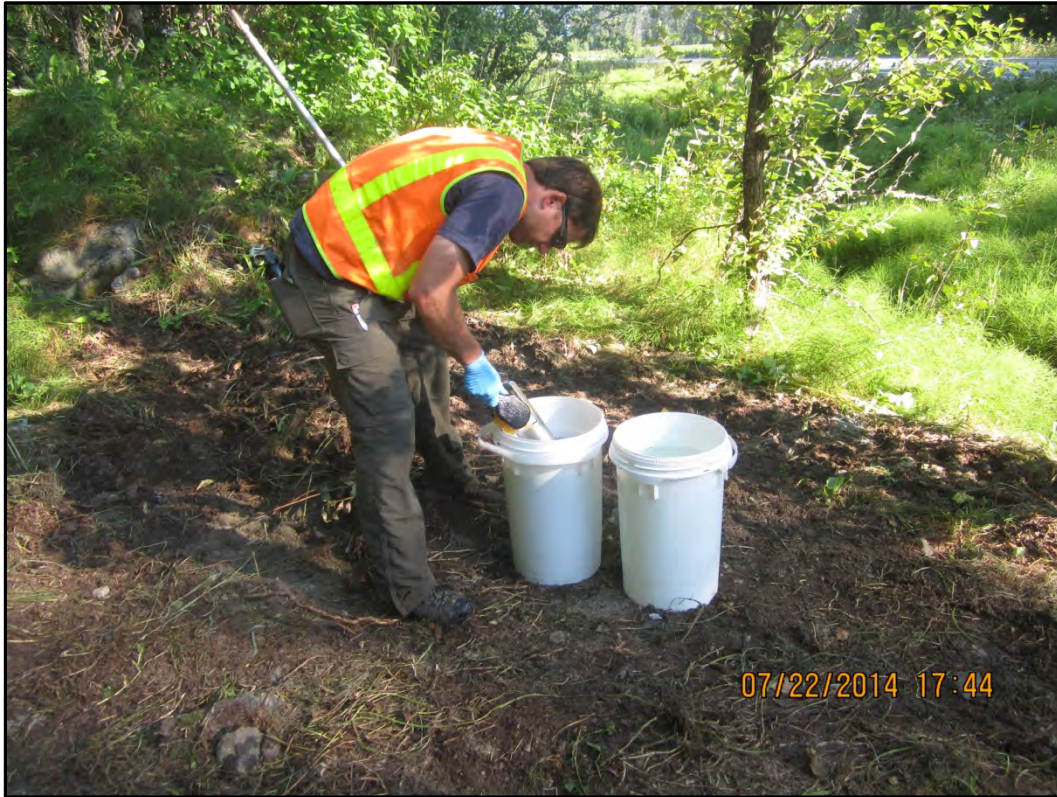
Photograph 19 – Sediment collection equipment was decontaminated with alconox and rinse water after each sample was collected. View to the south.
