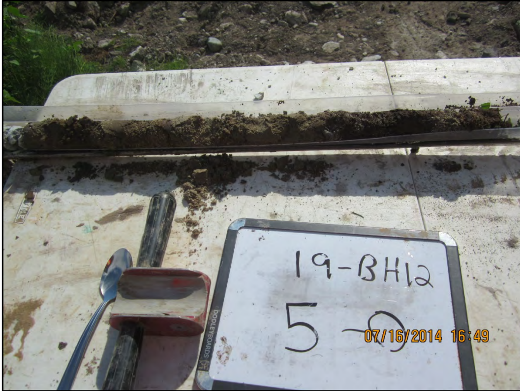
Photograph 23 – Soil lithology from boring 19-BH12 between 0-5 feet bgs. Silt with organics, silty sand, brown and dry.
