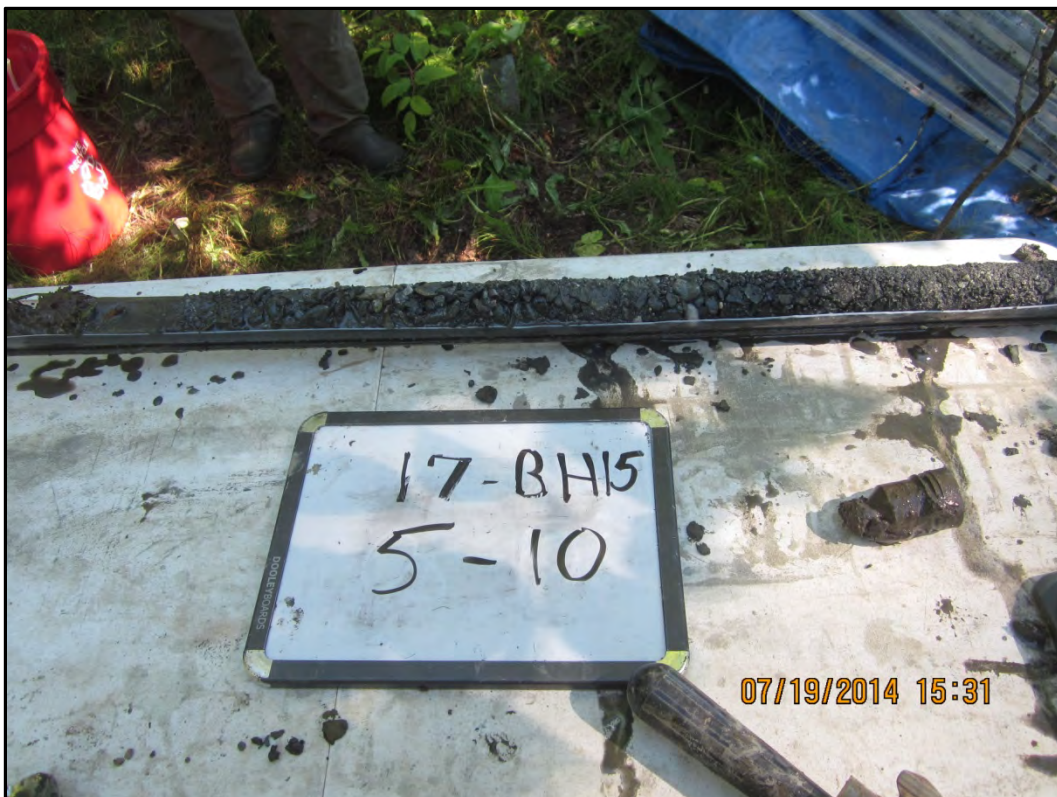
Photograph 6 – Soil lithology from boring 17-BH15 between 5-10 feet bgs. Silty gravel, gray, saturated. PID readings up to 1,015 ppm; sample collected from 9-10 feet bgs.
