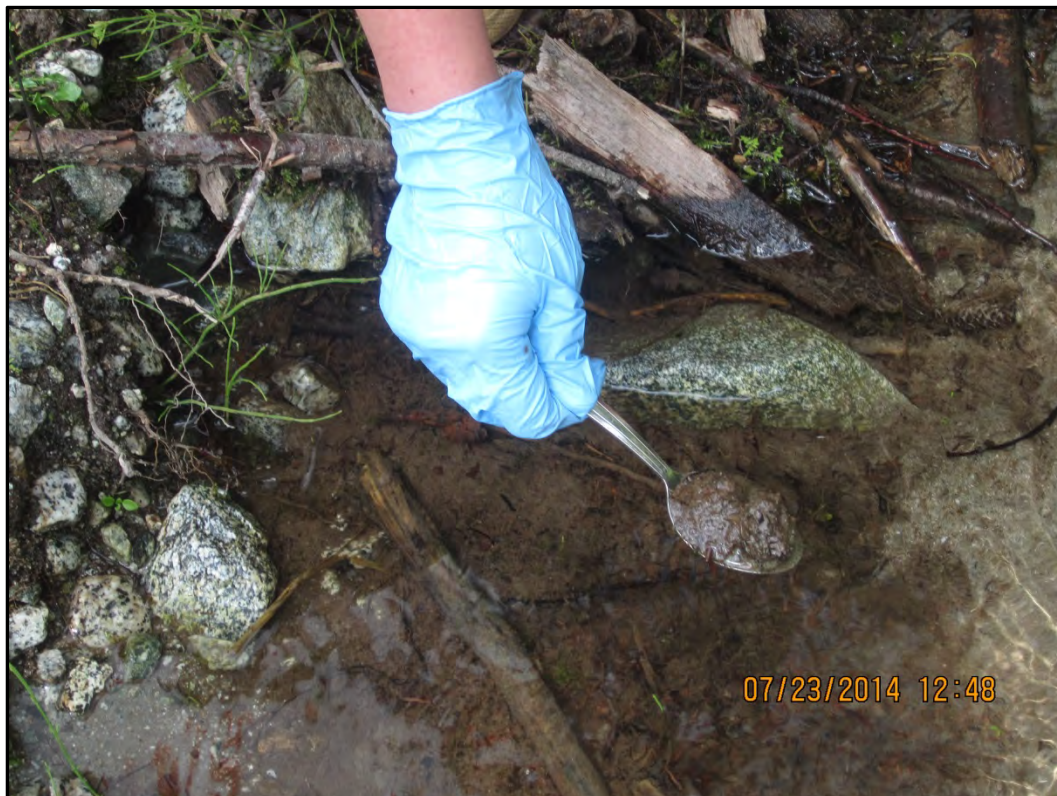
Photograph 32 – Collecting a sediment sample (19-SE1) with a stainless steel spoon during the initial sampling event in July; these samples were all re-collected in August due to elevated cooler temperatures.
