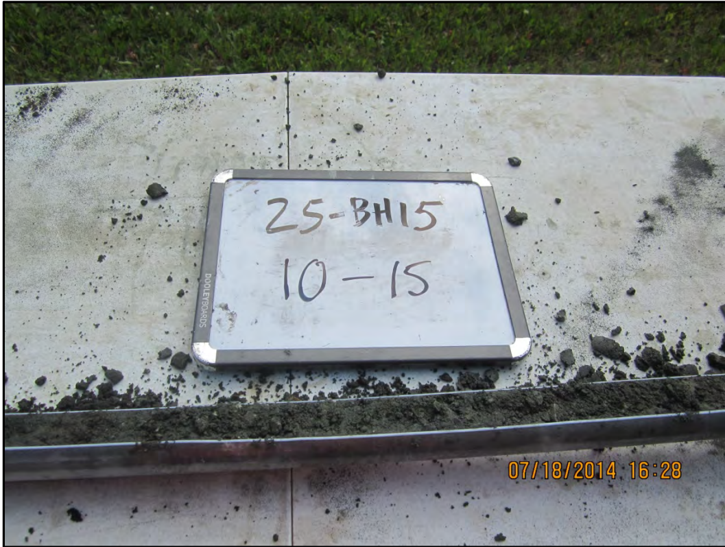
Photograph 43 – Soil lithology from 25-BH15 from 10-15 feet bgs. Sandy silt with gravel, gray and black, dry.
