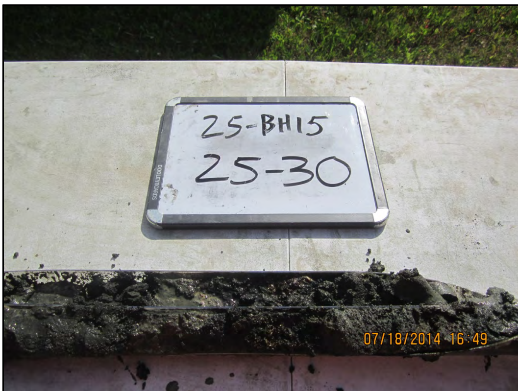
Photograph 46 – Soil lithology from 25-BH15 from 25-30 feet bgs. Silty sand with gravel, gray and black, saturated. Sample collected from 25-26 feet.
