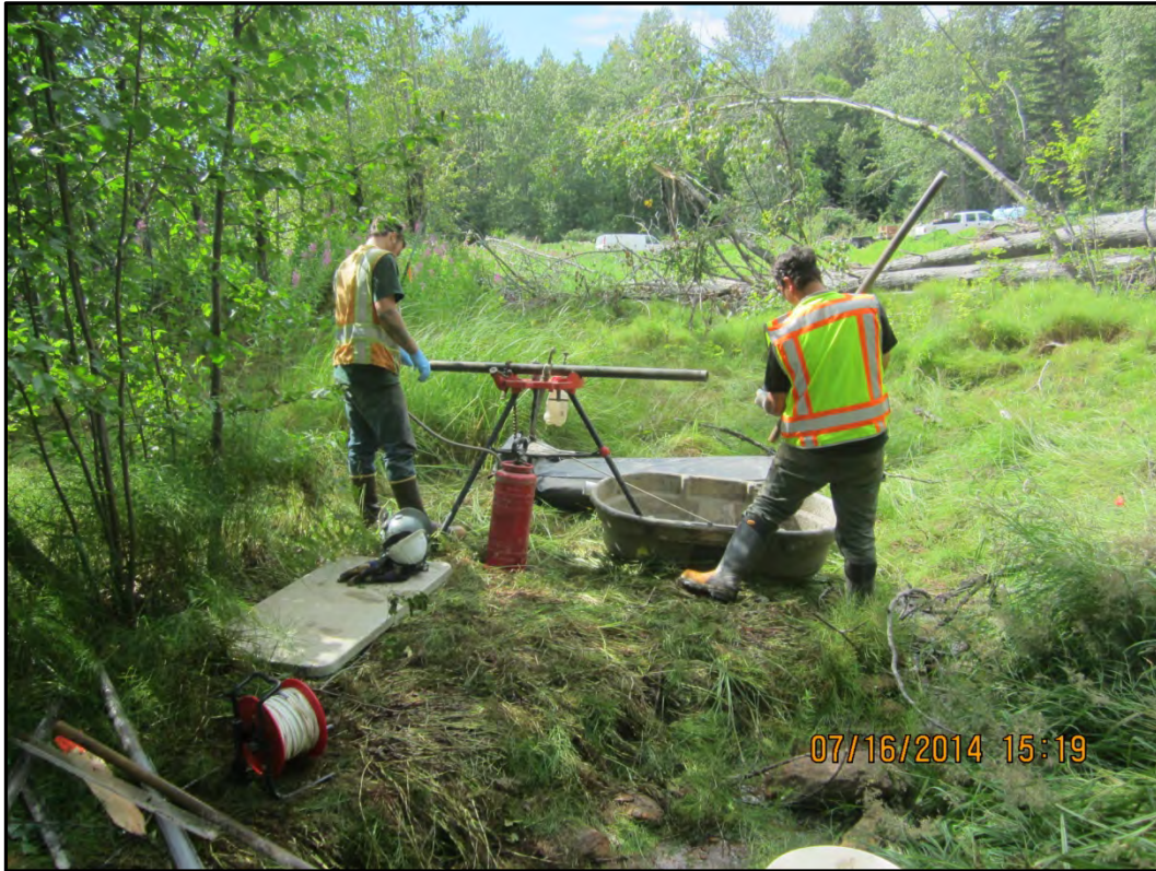
Photograph 27 – Decontamination of drill rod at PMP19.5, near 19-MW1/BH08. View to the northwest.
