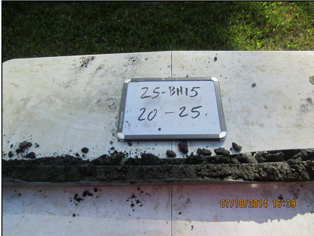
Photograph 45 – Soil lithology from 25-BH15 from 20-25 feet bgs. Silty sand with gravel, moist at 20 feet wet below 23 feet.
