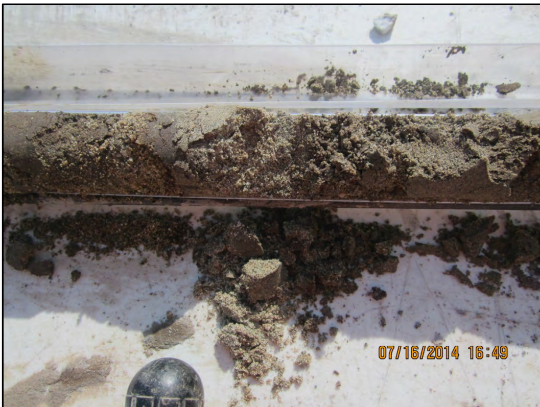
Photograph 24 – Close-up of soil lithology from boring 19-BH12 between 0-5 feet bgs.
