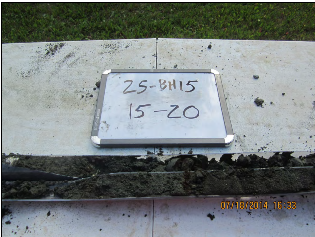
Photograph 44 – Soil lithology from 25-BH15 from 15-20 feet bgs. Sandy silt with gravel, silty sand with gravel, and crushed white rock layer. Moist at 20 feet.
