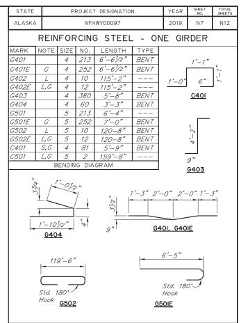
E - Epoxy coat all Girder reinforcing
