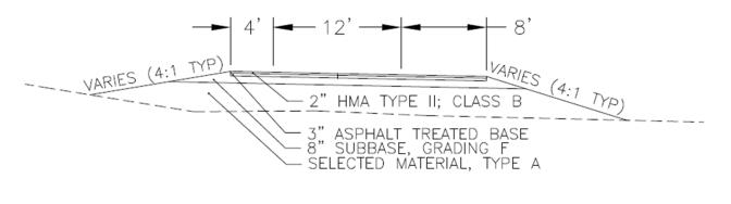
TYPICAL SECTION ON AND OFF RAMP Figure 3c.
