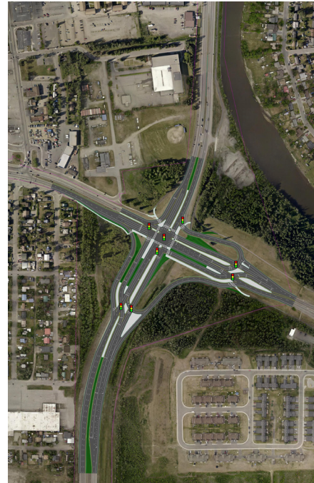
Continuous Flow Intersection Median U-Turn (CFI-MUT)
