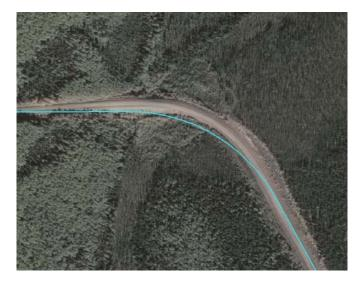
Then, Fix Grades (due to the ice-rich nature of the existing roadway, a balanced cut/fill profile is not a viable alternative)
