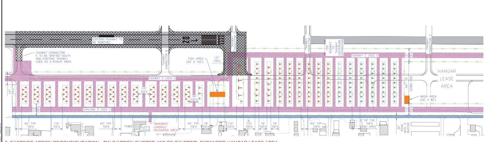
2. EASTSIDE APRON RECONFIGURATION - TW C/APRON SHIFTED 150' OF SKI STRIP, EXPANDED HANGAR LEASE AREA
